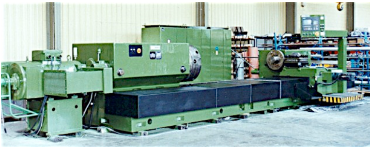
Heckert Roll lathe, reconditioned and retrofit for Gear & Shaft by Acumat and CNC Design.
