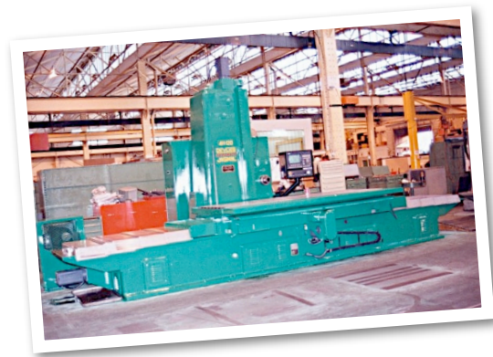
One of three Herbert De Vlieg Jig borers reconditioned and CNC retrofit by Acumat and CNC Design.
